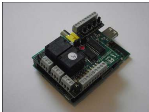
FIGURE 11-13: The buffered outputs of the PiFace mean you can control far more without worrying about the small current limits on the Raspberry Pi.
